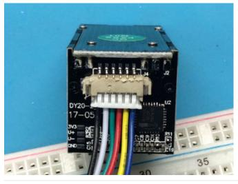
If your sensor has different wires, The first wire from the left should be the black wire ground, then the two data pins, RX is the white wire, TX is the green wire then the red power wire. You'll have to cut, strip and solder thicker gauge wires to the current wires.
